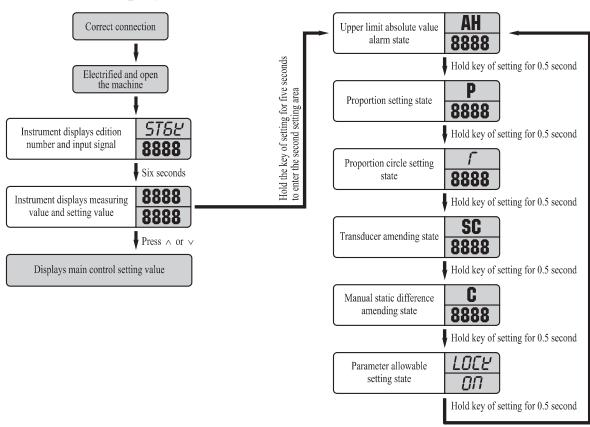
The operation of the instrument with main control way of digit type
